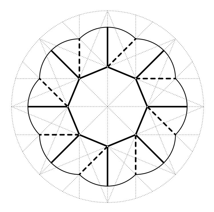
This pattern can be used to make a small coin purse out of leather. The result is a flat, octagonal construction that fits well in a pants pocket and will keep the pocket from being worn through by loose coins. Use a piece of leather six inches in diameter, not too thick but stiff enough to hold its shape. 0.40" is about right. Transfer the pattern to the leather, cut, crease, and fold as shown, and press wet overnight to set the shape. Make a sample by folding a copy of the pattern itself.
